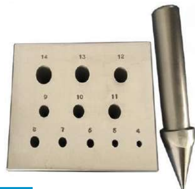
VI -499 Bezel Block Oval Shape Hole with 17 Degree Punch
