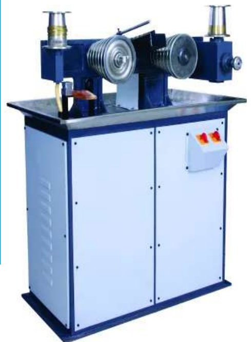
VI -718 Wire Drawing Machine Electric Available : Six Pass , Nine Pass & 12 Pass
