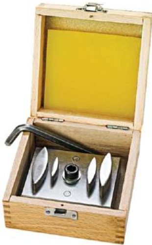
VI -488 Ring Blank Disc Cutter Set Of 4 with Wooden Storage Box
